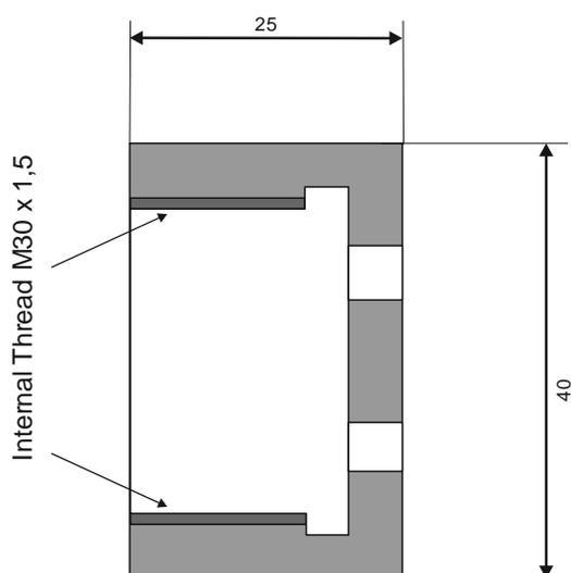
Fig. 1 Dimensions of the cap
